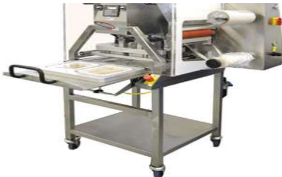
Figure 19 : Modify atmospheric packaging
